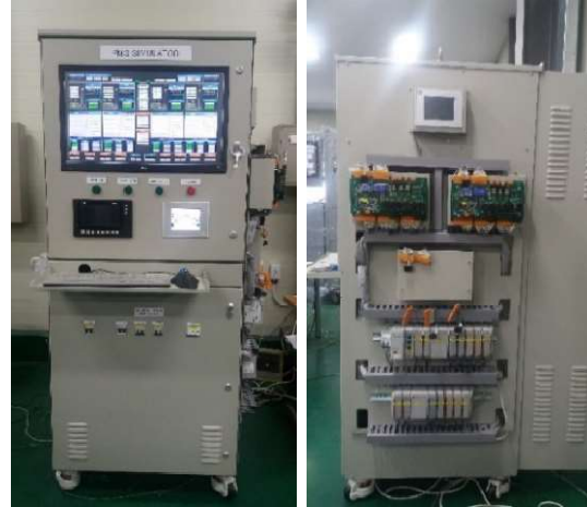
Figure 12: PMSIM-V2: PMS simulator with PMS unit for test
