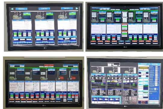
Figure 13: Operation HMI screens of PMSIM-V2 (3 DG, 4 DG with special function, shaft generator, and WHRS)
