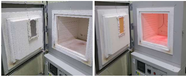
Figure 2: Installation of the test specimen in heating furnace
