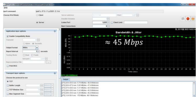
Figure 5: Communication channel bandwidth ((a) Test setup, (b) Measurement result)
