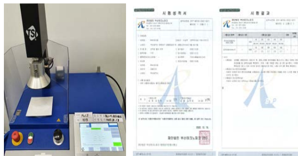
Figure 3: TSI 8130 filter media tester and performance evaluation certification for filter materials
