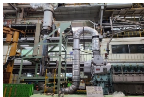
Figure 5: Experiment facility, STX-MAN diesel engine.
