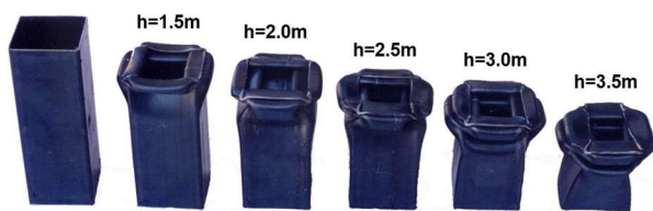
Figure 4: Test specimen after the drop test for drop height
