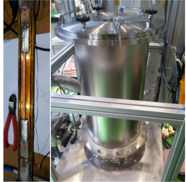
Figure 7: System used for measuring the critical current of the HTS tape according to the operating temperature and external magnetic field
