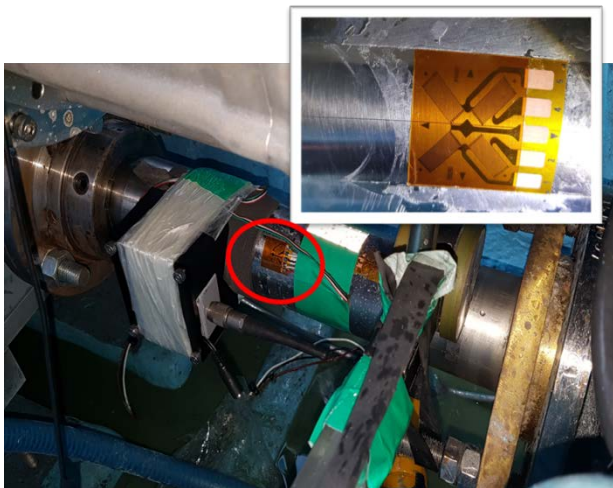
Figure 4: Strain gauge and telemetry system installation at the propeller shaft for torsional vibration measurement
