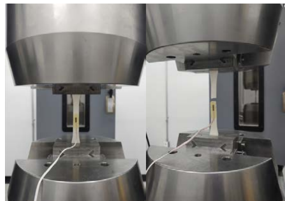
Tensile tests (b) before break and (c) after break
