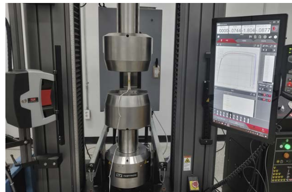
(a) Setup used for the tensile test for biodegradable plastic materials
