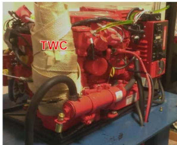
Figure 1: Photograph of stoichiometric engine bench for exposing TWC to lubricant additives
