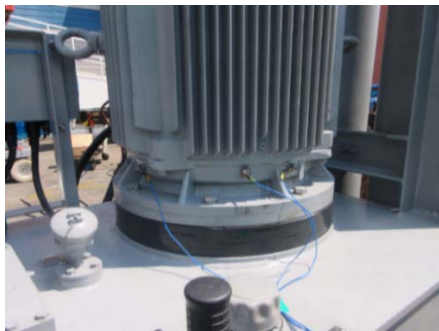
Figure 8: Measurement position of motor bearing casing
