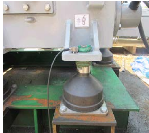
Figure 5: Accelerometer on top of mounting
