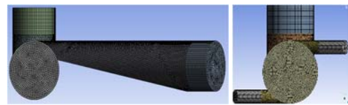
Figure 4: CFD meshing of two Inlet Nozzles on GLCC
