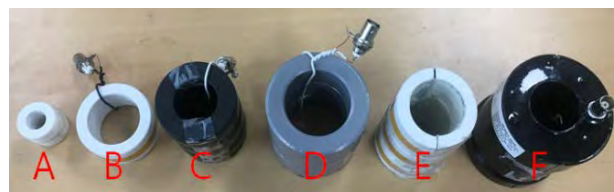
Figure 3: Inductive coupler using a soft magnetic core
