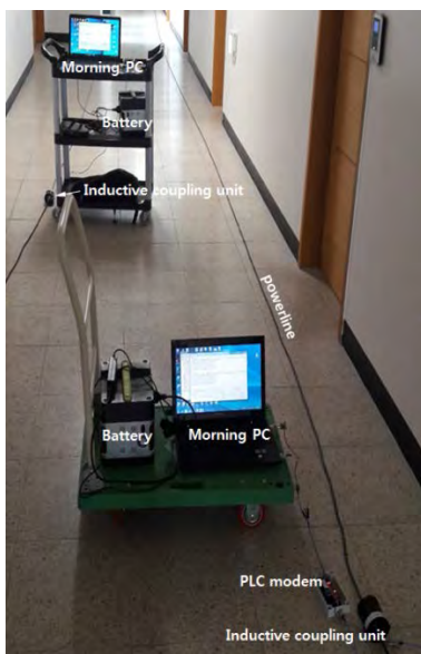
Figure 10: Communication performance measurement setup
