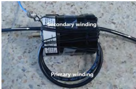
Figure 7: Inductive coupler with turns ratio of M:N
