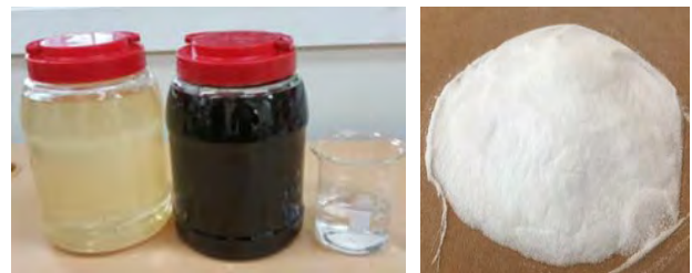
Figure 1: Basic raw materials of polyurethane foam (Polyol, isocyanate, blowing agent) and glass bubble
