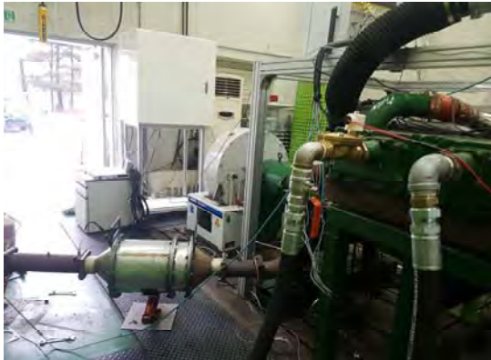
Figure 2: Image of the D6CB engine and the DPF
