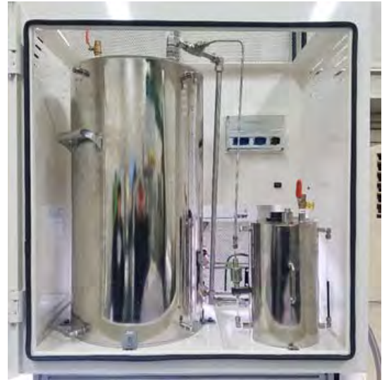
Figure 1: Image of the fuel borne catalyst supply device
