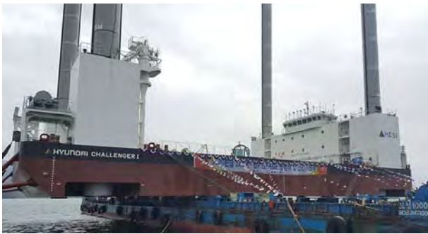
Figure 1: Jack up barge employed for analysis
