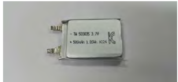
Figure 4: Lithium polymer battery
