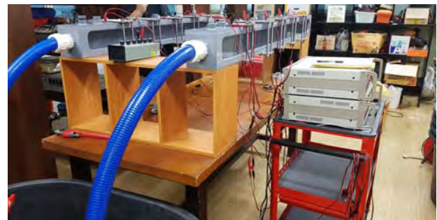
Figure 1: Schematic drawing and appearance of cooling seawater pipe experimental equipment with the ICCP system
