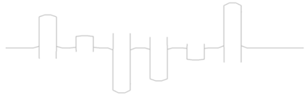
Figure 5: 1D FE model of crankshaft
