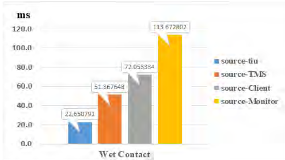
Figure 4: Assuming that data is generated in the application layer, the average transmission time from the wet contact to each destination
