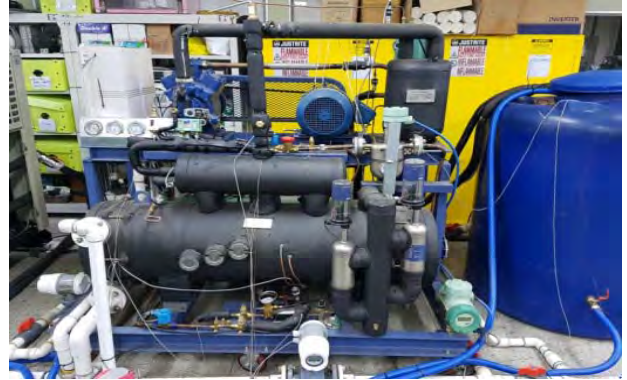
Figure 1: Experimental apparatus of the seawater cooling system
