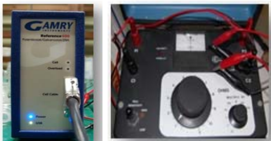
Figure 4: View of potentiostat(left side) & resistivity meter(right side)
