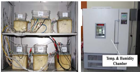
Figure 3: View of mortar specimens in temperature & humidity chamber
