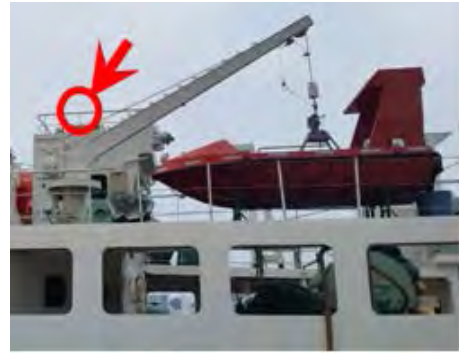
Figure 2: Side view of ship's winch room. The pyranometer was installed on a structure at the side of the ship's winch room
