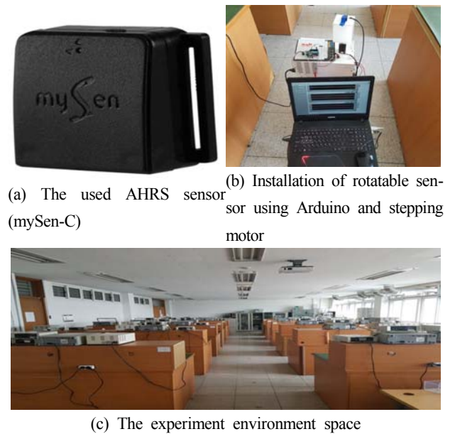
Figure 6: The AHRSS sensor and module used for experiment and experimental condition
