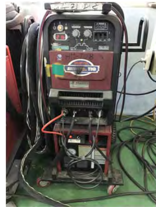
Figure 9: 600 A class arc welding machine for shipbuilding
