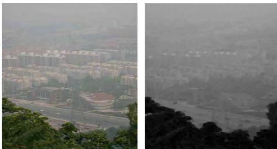
Figure 2: dark channel evaluation (a) input fog image (b) dark channel of (a) by 15x15 window
