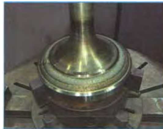
Figure 6: GMAW, Seating surface with Inconel 718
