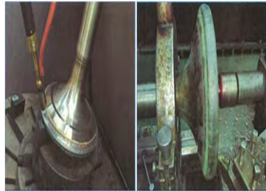
Figure 5: GMAW, Bottom & side with Inconel 625
