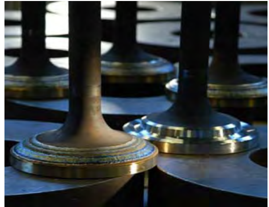
Figure 1: Photo of exhaust valve spindles
