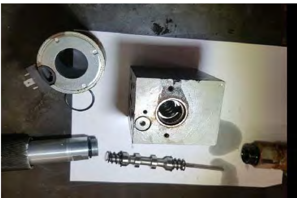
Figure 9: Disassembly investigation of clutch control solenoid valve
