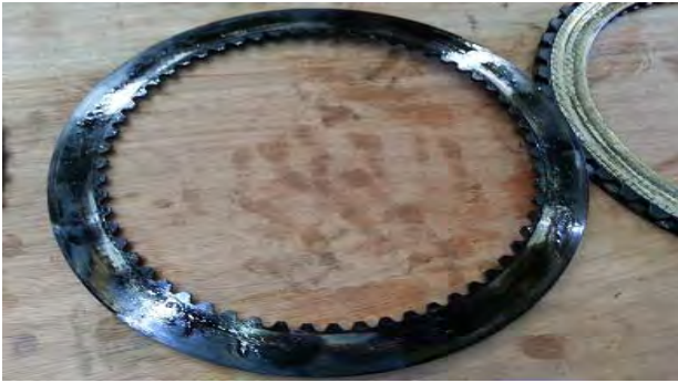
Figure 7: Damaged pair of inner and outer plates
