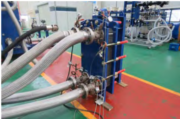
Figure 3: Thermal performance test of Hybrid plate heat exchanger
