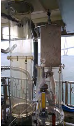
Figure 4: Reduction catalyst for pilot test
