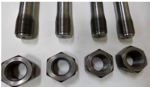
Figure 11: U nuts for connecting rod bolt on board
