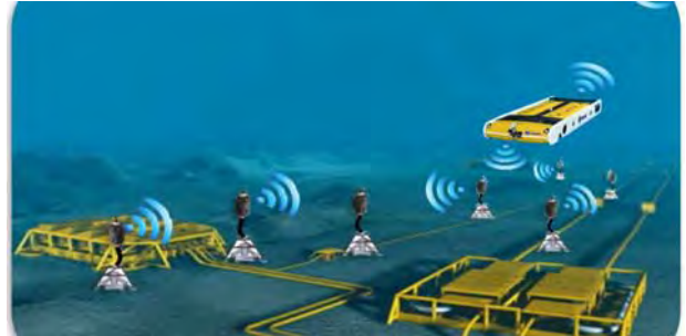
Figure 2: Example of underwater multiple sensors acoustic communication
