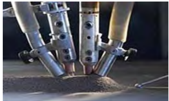
Figure 1: Tandem SAW torch [2]
