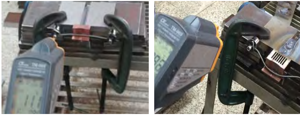
Figure 4: Measurement of the temperature variation of two types of end-tab using non-contact thermometer during and after the time heat is applied
