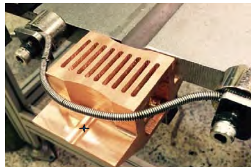
Figure 3: Indication of the location where temperature variation of end-tab is measured. (indicated by a black cross point)
