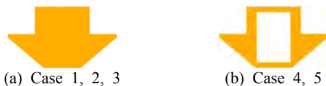
Figure 7: Classification of two types of end-tab according to the existence of the parallel hole
