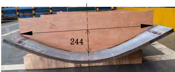
Figure 2: Template for curved surface check
