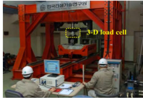
Figure 2: Conventional method for cutting force measurement with a 3-D load cell (redrawn from [2])
