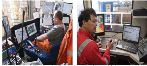
Figure 6: Cyber base(Driller cabin)
