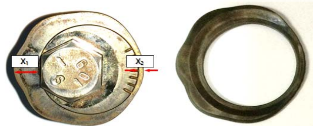
Figure 3: Dimension and shape of chip after trimming process
