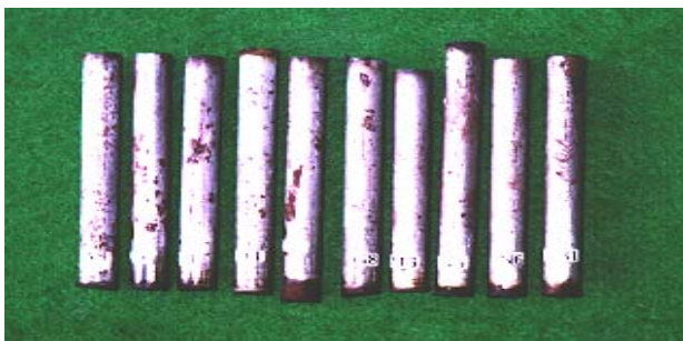
(a) rebar surface of 40 mm cover thickness
