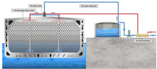
Figure 6: Concept design of cargo hold for regasification in NGH pellet carrier
