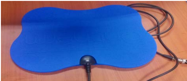
Figure 16: Manufacturing of the insulated earth plate
