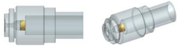
Figure 6: 3D modelling of full cone type nozzle
