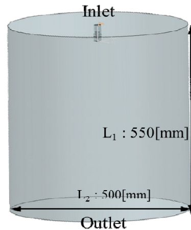
Figure 7: 3D modeling of Scrubber (single nozzle)
