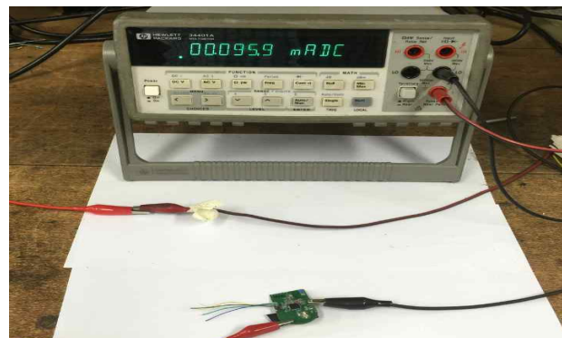
Figure 5: Current measurement at power down mode
