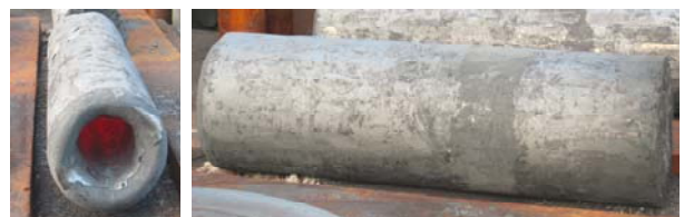
Figure 12: Forging product under still air cooling
