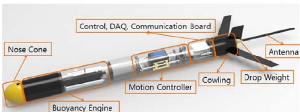
Figure 1: Configuration of underwater glider
