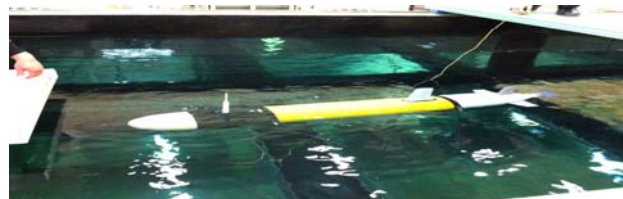
Figure 7: Measurement of the drag force of AUV
