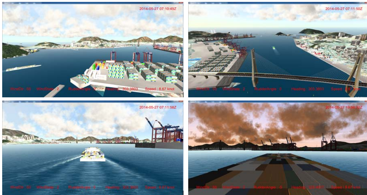
Figure 16: Navigation environment and views of the created 3D terrain visualization system
