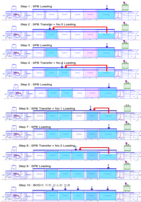
Figure 5: LNG operation procedure
