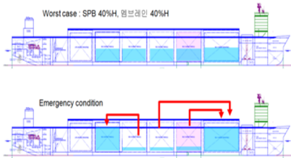
Figure 7: Emergency LNG transfer (Combined containment system)
