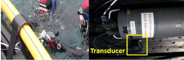
Figure 9. Sensor module with underwater communication modem
