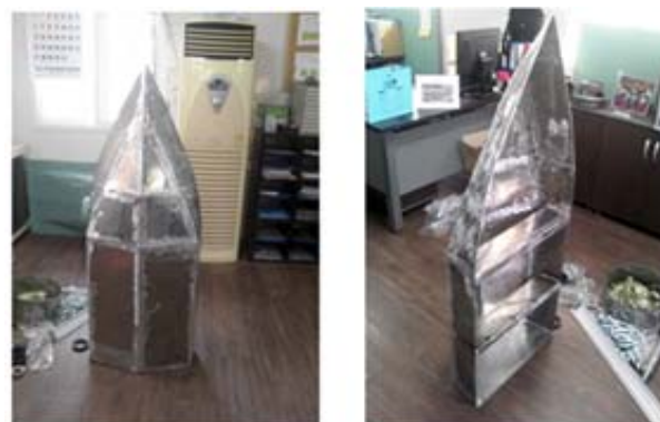
Figure 14: Actual prototype image for Al 5083 co-environmental boat discussed in this study
